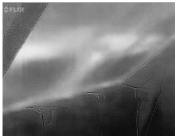
Missing insulation to roof void and pitch.
